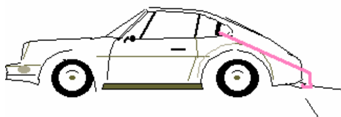
Figure 1. The experimental set up for exhaust gas collection
