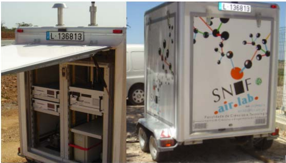
Figure 1: Aspects of the interior and exterior of the mobile laboratory - SNIF AIRLAB and its measurement equipment
